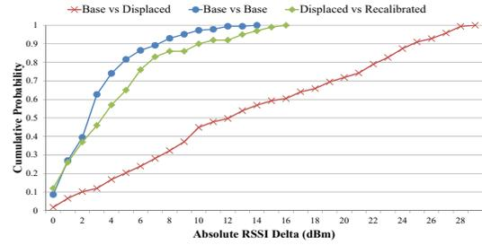
Fig. 3: Probability distribution of absolute RSSI delta of one access point in Office environment
