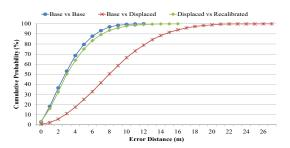
Fig. 5: Localization error distribution for displacement of half the deployed signal sources in Warehouse environment
