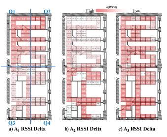
Fig. 2: Average RSSI delta per cell for displaced access points
