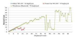
Fig. 1: Displaced vs Detected signal sources in different environments
