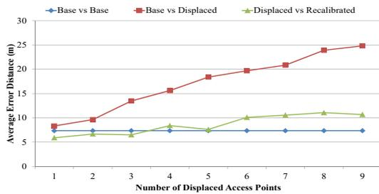
Fig. 6: Localization performance comparison over successive displacements in Trade Fair Environment
