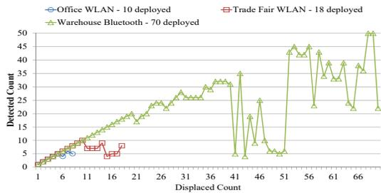
Fig. 1: Displaced vs Detected signal sources in different environments
