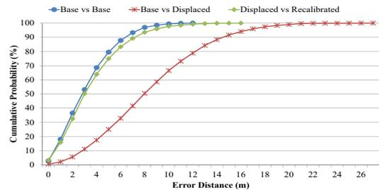
Fig. 5: Localization error distribution for displacement of half the deployed signal sources in Warehouse environment
