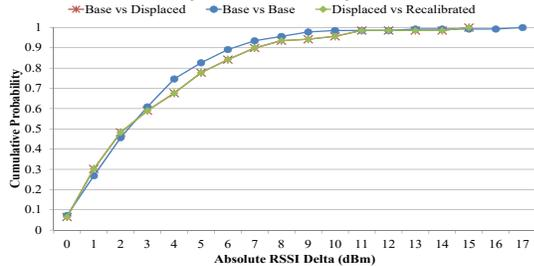
Fig. 4: Probability distribution of absolute RSSI Delta after recalibration of false positive detection
