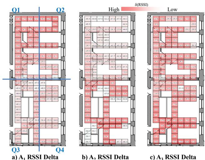
Fig. 2: Average RSSI delta per cell for displaced access points
