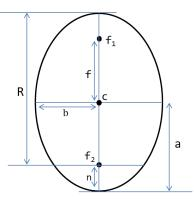
Figure 2. Properties of an ellipse
