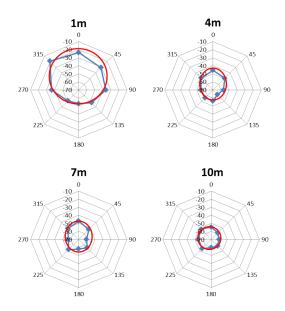
Figure 1. Signal distribution (in dBm) with distance
