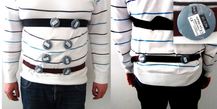
Figure 12: Tag placement on t-shirt (loose) and with belts (tight)
