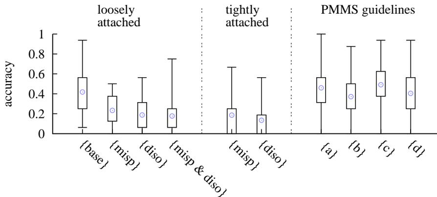
Figure 13: Localization accuracy for single tags
