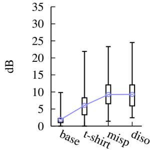
Figure 7: Signal strength variability (with human body)
