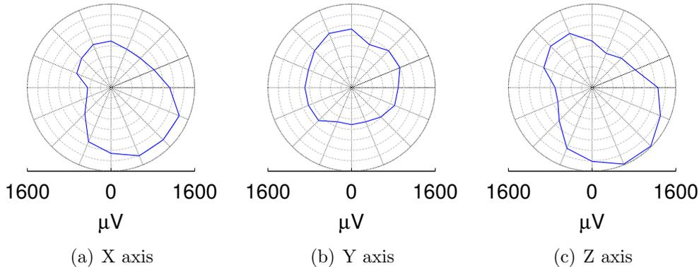
Figure 2: Antenna radiation pattern measured at 1m for the different axes
