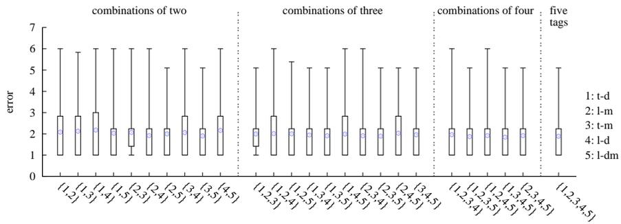
(a) Localization error for multiple tags that are misplaced and/or disoriented
