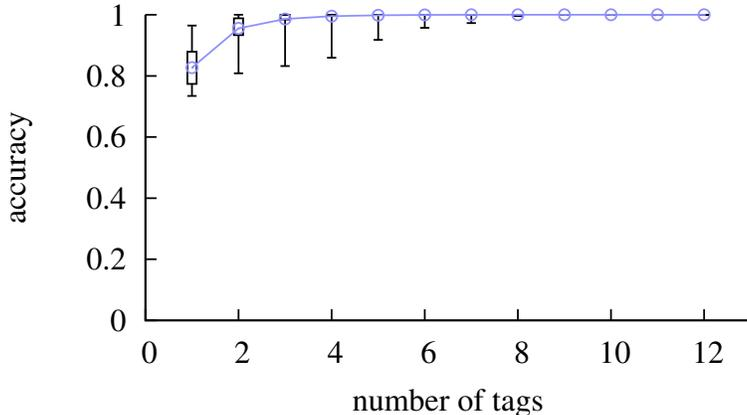
Figure 10: Localization accuracy of multiple tags on human body
