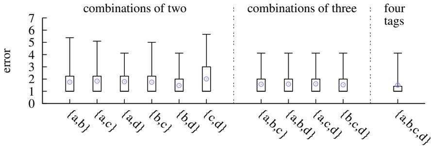
(b) Localization error for multiple steady tags following the PMMS guidelines
