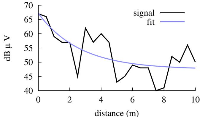
Figure 3: Signal strength vs. distance in an aisle
