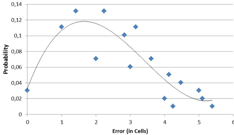
**Fig. 2.** Localization error probability distribution in the lab
