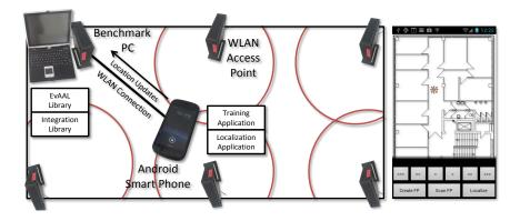
Fig. 1. Basic Deployment (left) and Training Application (right)
