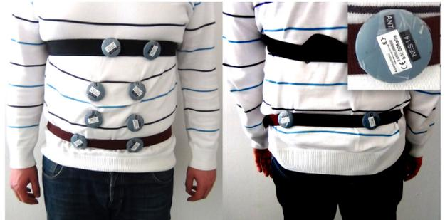
Figure 11. Tag placement on t-shirt (loose) and with belts (tight)
