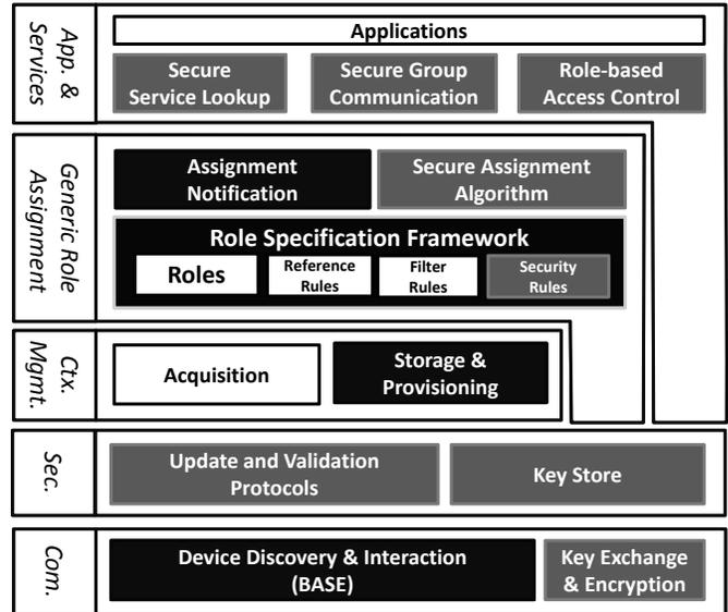
Fig. 3. Secure Role Assignment System Architecture
