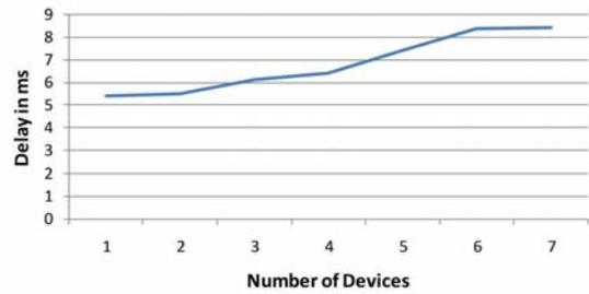
Fig. 8. Latency for Reference Rules with Varying Number of Devices
