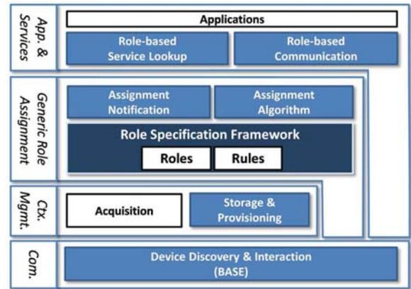
Fig. 2. Generic Role Assignment System Architecture.
