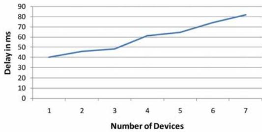
Fig. 7. Latency for Filter Rules with Varying Number of Devices
