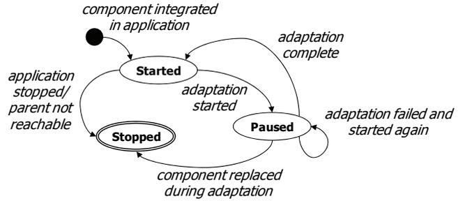
Fig. 3. Extended Component Lifecycle
