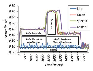
Figure 4. Decomposed Power Usage
