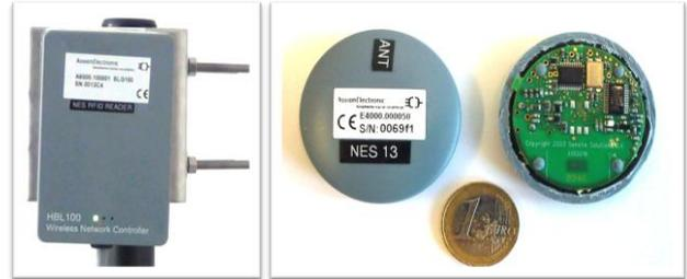
Figure 2: LogiSphere RFID Reader and Tags
